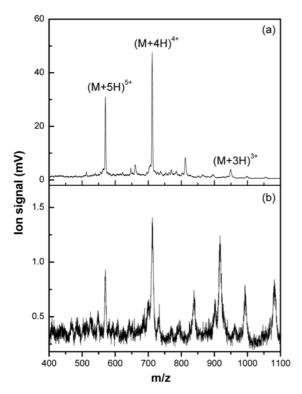
**Figure 2**. Mass spectra of melittin ions produced by ESI (a) with and (b) without helium gas in the ion trap. The pressure of the main chamer increased to  $5 \times 10^{-4}$  torr with the helium gas.
