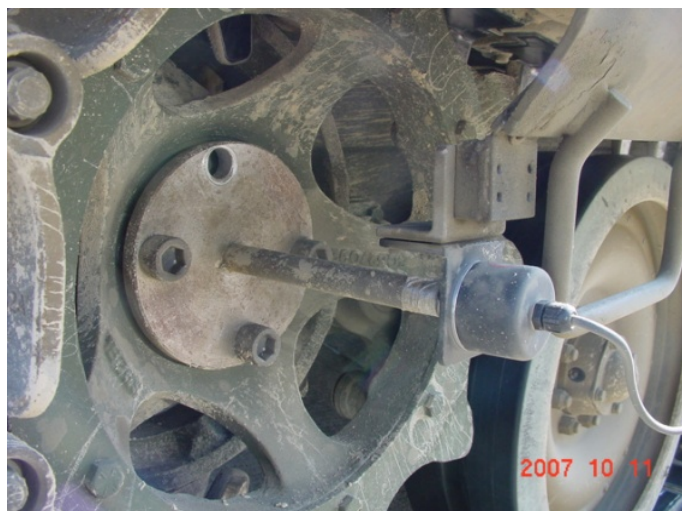
Figure 3. Tacho-generator for the engine RPM measurement.
