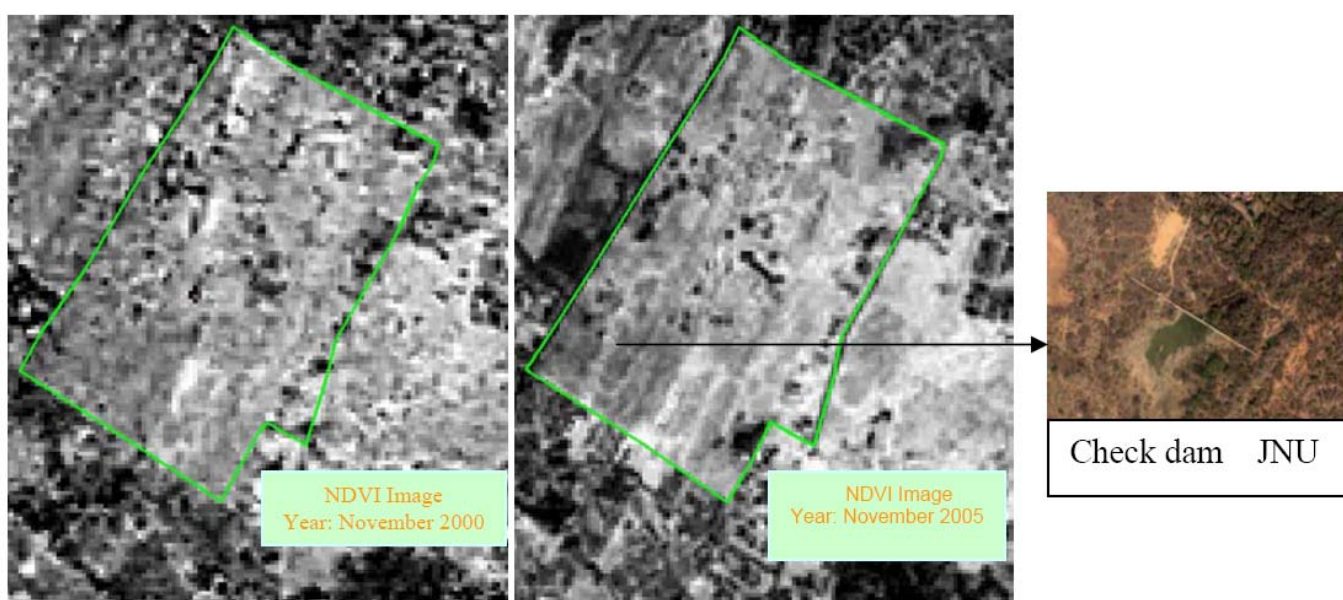
Figure 4. Change in NDVI study by IRS-1D LISS-III and PAN sensor data showing more vegetation as black patch in JNU, a part of Aravalli Quartzite ridge in New Delhi, India. This data was used for selection and monitoring of groundwater recharge (check dam).
