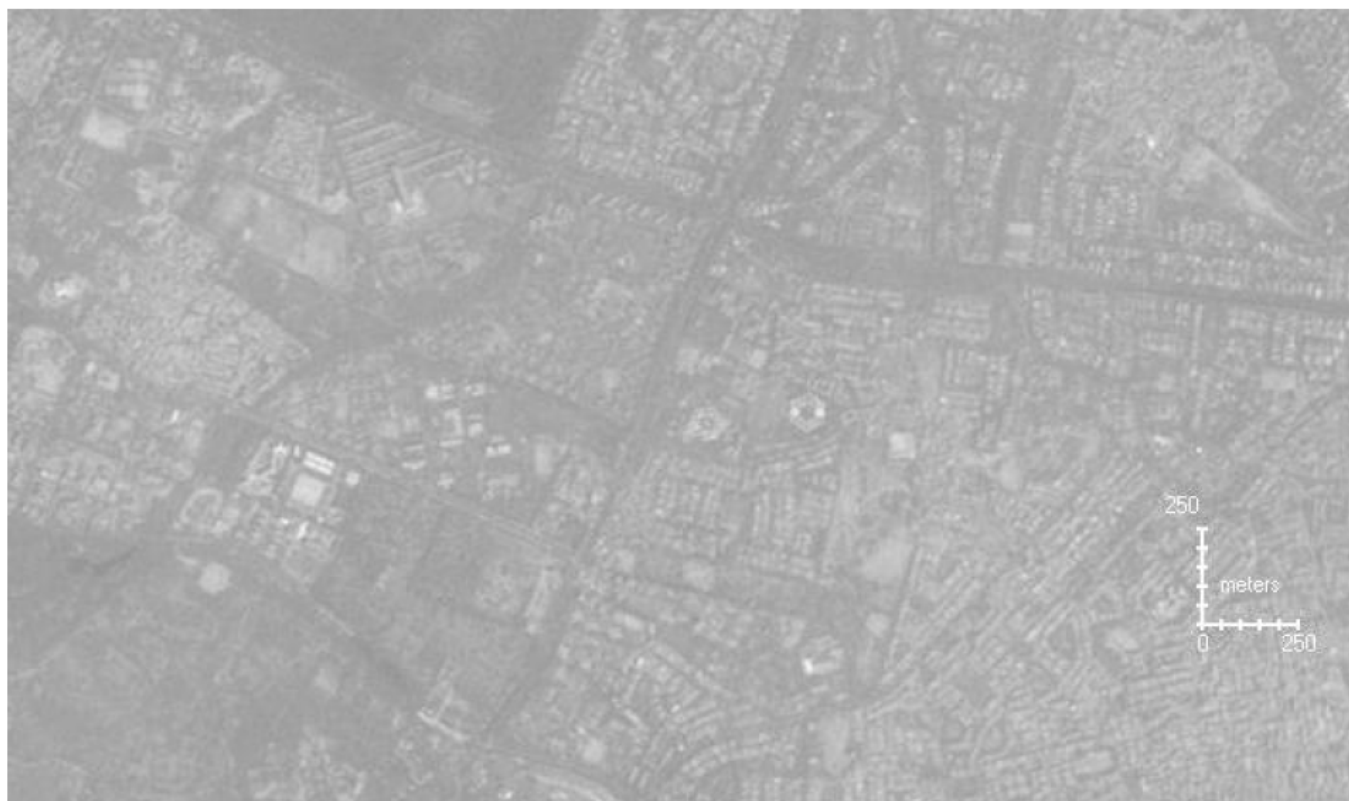
Figure 3. IRS-1D Panchromatic sensor data using ERDAS software showing detailed landuse useful in pinpoint location of groundwater recharge points.
