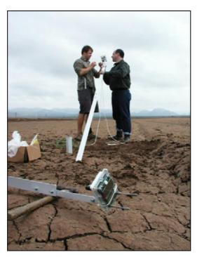
**Figure 5.** NASA/JPL team members deploy a Sensor Web 3.2 pod in recharge basin. Extended stands allow the pods to stay operational above water during a flooding event. Note polygon patterns in soil, indicative of previous flooding/drying cycles.
