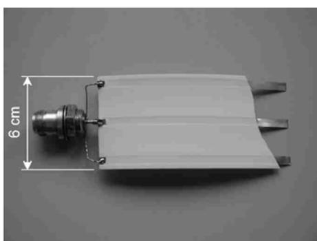
The electrical field concentrates around the conductors and defines the sensitive area of 3 to 5 cm around the cable. The spatial weighting of the measurements in the cross section of the cable is directly related to the energy density distribution. The electric properties of the cable can be calculated and measured. One can assume that the well-known equivalent circuit for the infinitesimal line section as shown in Figure 4 fully describes the electric properties of the line.
