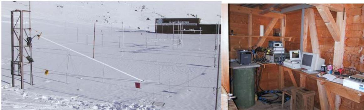
The natural settling of the snow cover was reflected nicely in the horizontal cable measurements (Figure 12). The measured increase of snow density was in accordance with manual measurements. It increased from initially 100-200 kg m<sup>-3</sup> to approximately 500 kg m<sup>-3</sup> at the end of the winter season.
