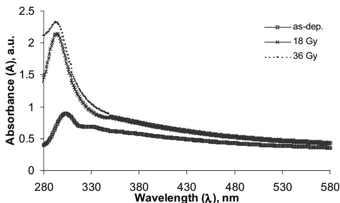
**Figure 2.** The absorption spectra for as-deposited and irradiated 50 nm TeO<sub>2</sub> thin films.
