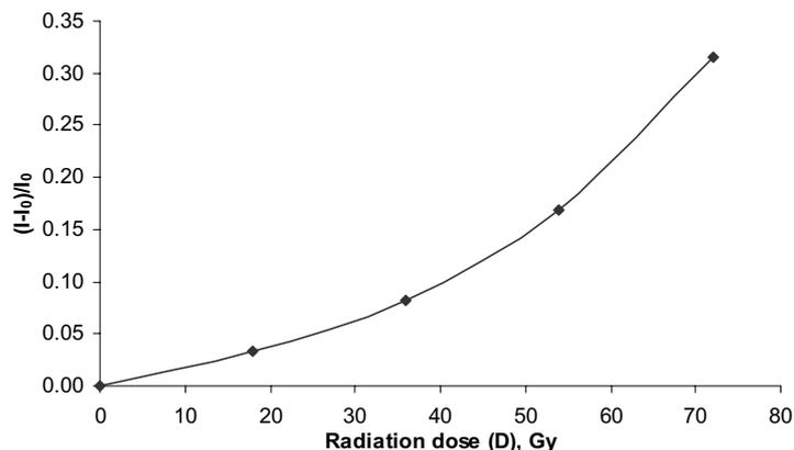
**Figure 6.** Dependence of the normalized current  $(I-I_0)/I_0$  versus radiation dose under an applied voltage of 2 V for  $\text{TeO}_2$  thin films.
