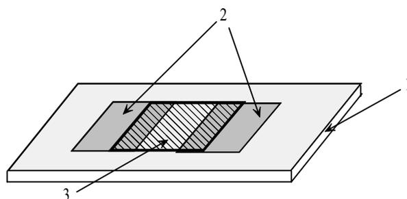
**Figure 1.** Planar structure used for the electrical parameters measurements, where 1 is a glass substrate, 2 – Al layers used as electrodes, 3 – layer of  $\text{TeO}_2$
