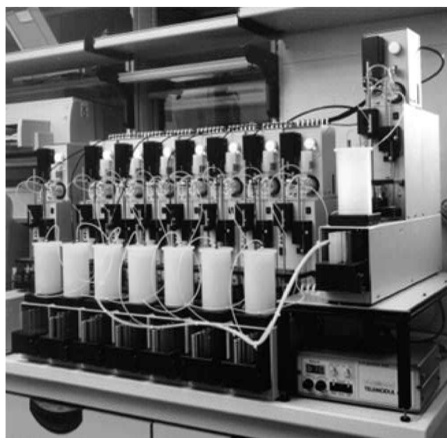
Figure 10. The modified Zymark RapidTrace® SPE workstation developed for single-step and multi-step SPE fractionation and concentration.
