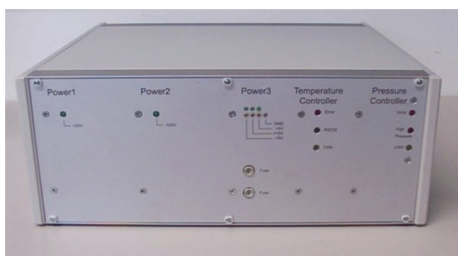
FIGURE 6: Electronic equipment rack.
