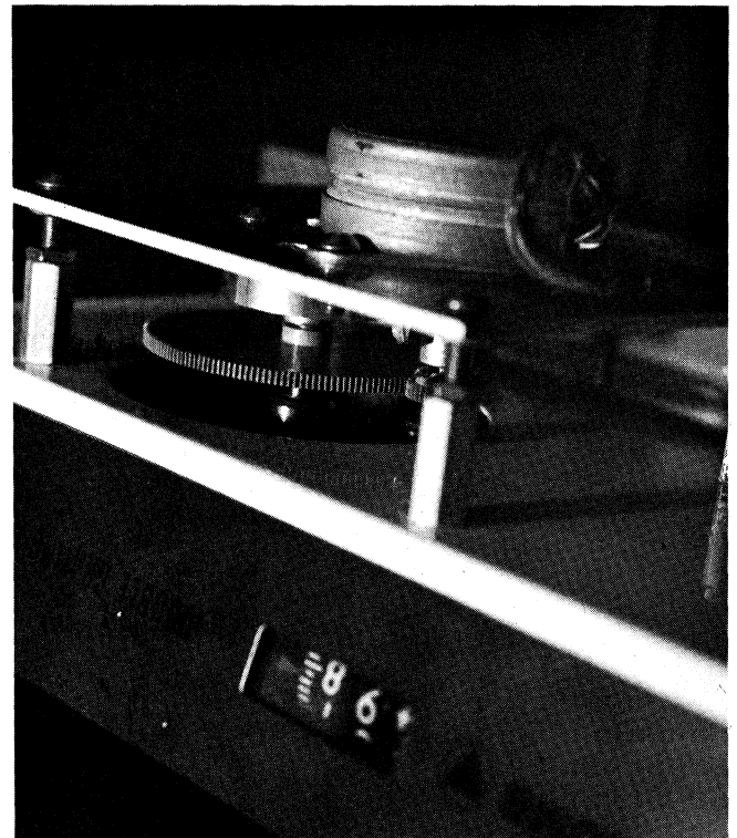
Figure 4. Photograph of the stepper motor monochromator drive assembly.
