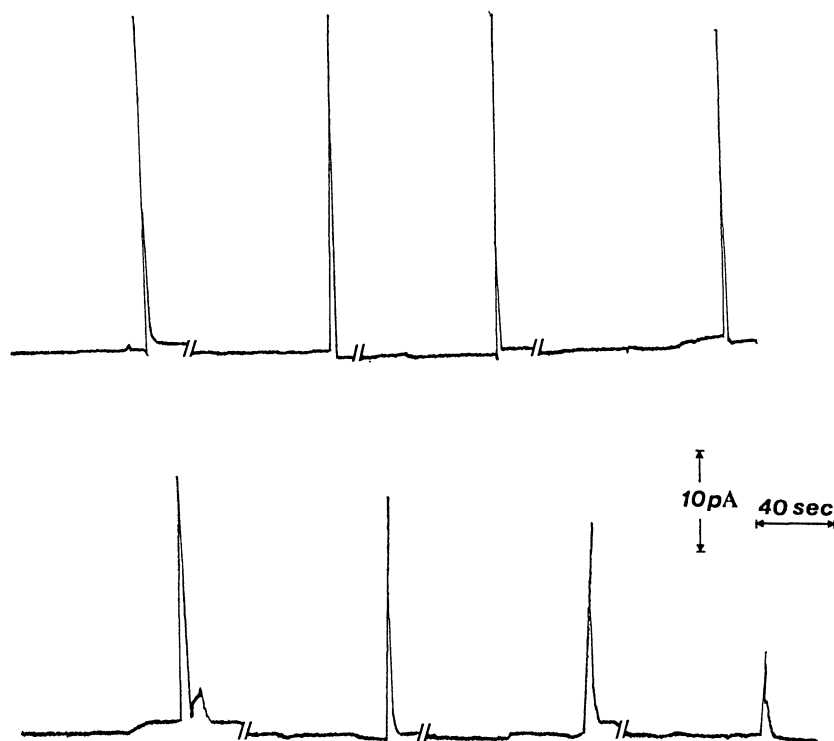
Figure 6. Signals obtained during a cycle of repetitive injections of 3.50 \times 10^{-7} M T4 at pH 6.0 (0.1 M KCl, 10 mM HEPES and in the absence of \text{Ca}^{2+} ) with BLMs composed of 15% (w/w) DPPA when 3 \mu\text{l} of solution containing 0.62 mg/ml antibody was co-deposited onto the air/electrolyte interface. The time delay between the repetitive injections (marked as || in the figure) was 5 min.
