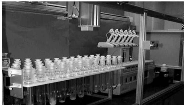
Figure 7. Automated system for focused microwave digestion of samples
