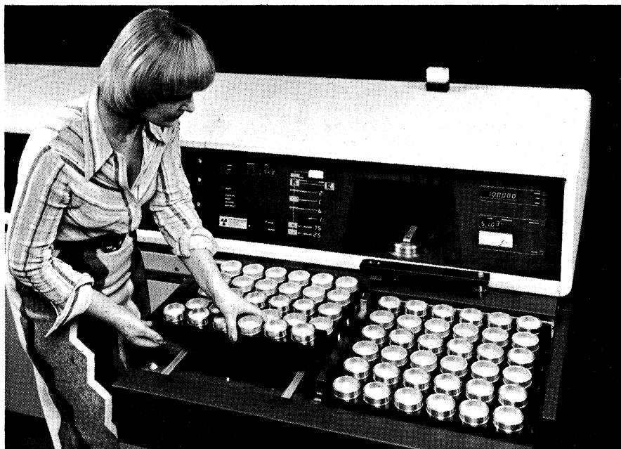
Operator removing a sample tray from the automatic sample changer of the Philips PW1400 sequential XRF spectrometer.
