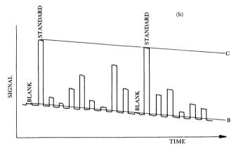
Figure 2. Flame AAS traces indicating assignment of base-line (B) and calibration (C) by an instrument microprocessor (figure 2[a]) and an external microcomputer (figure 2[b]).
