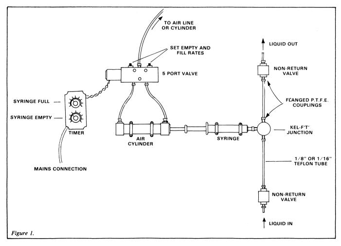
period during which the valve is either on or off and the rate of pumping. An air supply from a cylinder or air line at a pressure of a few kilograms per square centimetre is required.
