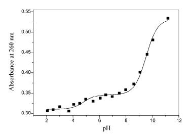
Figure 2. The spectrophotometric titration curve of 0.08 mM 3 at 260 nm in 20% vol. MeCN.
