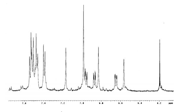
**Figure 1.** Aromatic region of the <sup>1</sup>H NMR spectrum of macrocycle **3** in CD<sub>3</sub>OD (see Experimental Section for signal assignments).
