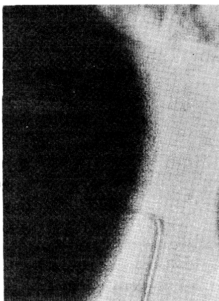
Figure 1. Acrylamide crystal irradiated by a collimated X-ray beam showing the edge of the irradiated region. Magnification 50X
