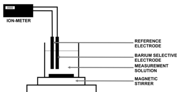
Figure 1. The potentiometric titration of sulfates' system
