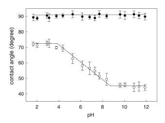
Fig. 3 Contact angle titration curves of the untreated PC surface (•) and of the PC surface treated with UV/ozone for 10 min( $_{\odot}$ )
