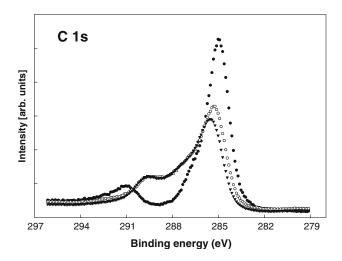
**Fig. 4** X-ray photoelectron C 1s signals of the untreated polycarbonate (•) and after the UV/Ozone irradiation for 10 min with mask on ( $\circ$ ) and without mask ( $\mathbf{v}$ ) on the surface
