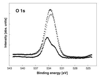
**Fig. 5** X-ray photoelectron O 1s signals of the untreated polycarbonate surface (•) and after the UV/Ozone irradiation for 10 min with mask ( $\circ$ ) and without mask ( $\bullet$ ) on the surface
