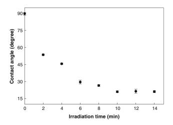
Fig. 2 The dependence of contact angle of the PC surface on UV/ozone irradiation time  $\ensuremath{\mathsf{UV}}$
