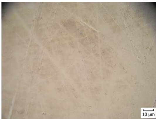
Fig. 4 Optical microscope image of Pd nanoparticles deposited onto Si substrate
