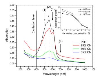
Fig. 2 Optical absorption measurements at room temperature of SWNT/P3HT composites as a function of wavelength. The *solid line* represents the initial excitation level at 400 nm. The vertical vectors represent the particular probing wavelengths of our transient absorption study. The inset shows the absorption peaks as a function of nanotube concentration at the singlet exciton transition and the vibronic sidebands
