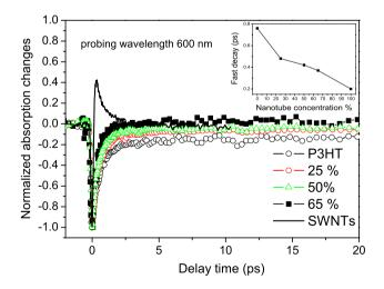
**Fig. 4** Normalized transient absorption measurements for the P3HT polymer, pure SWNTs, and SWNT/P3HT composites at probing wavelength of 600 nm. The inset shows the fast decay time as a function of nanotube concentration
