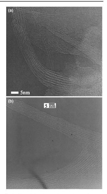
Fig. 1 High resolution electron microscopy images of (a) pure SWNTs and (b) SWNTs dispersed in P3HT polymer (SWNT concentration 50%)
