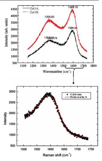
**Fig. 6** Raman spectroscopy on difference spots of the C–ZnO sample. The G peak has been re-drawn to show the asymmetry which is an indication of the phonon confinement in nanoclusters of carbon within the ZnO matrix
