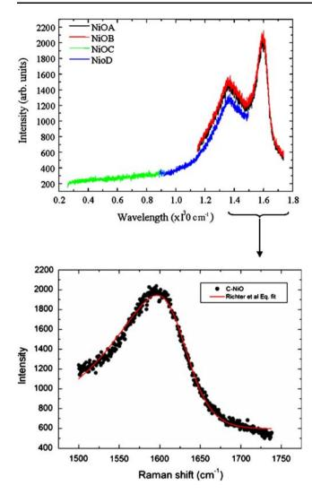
**Fig. 7** Raman spectroscopy on difference spots of the C–NiO sample. The G peak has been re-drawn to show that the carbon clusters are nanostructures as indicated from the asymmetry of this peak
