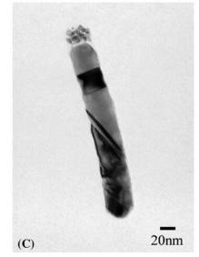
Fig. 6 TEM images of nanostructure with nanoparticles/dithiols junction between gold segments nanowire
