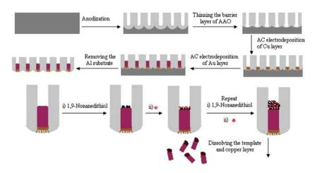
Fig. 1 Schematic diagram describing the fabrication steps of nano "cigars" based on the porous AAO template. Prior to the electrodeposition step, the thinning of the barrier layer is necessary to form the dendrite structure at the bottom. The copper as the first layer was electrodeposited and gold is then
