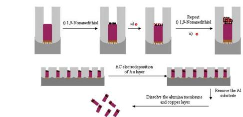
Fig. 2 Schematic diagram describing the fabrication steps of in-wire junction of nanoparticles by layer-bylayer assembly within the porous template carbon-coated copper mesh grid. All samples were examined in a JEOL 2000 EX TEM operating at 200 kV. The samples were all washed and centrifuged to remove the excess salt and surfactant prior to the characterization.
