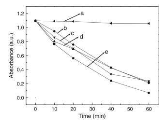
**Fig. 8** Plots of absorbance of Rhodamine B (detected at 553 nm) versus time under UV-light irradiation with (a) 0 g TiO<sub>2</sub>; (b) 0.02 g TiO<sub>2</sub>; (c) 0.02 g TiO<sub>2</sub>/H<sub>4</sub>TAPP<sup>6+</sup>; (d) 0.02 g TiO<sub>2</sub>/CoTPPS<sup>4-</sup>; (e) 0.02 g TiO<sub>2</sub>/porphyrin particles
