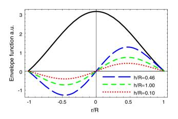
**Fig. 4** The first-order corrections (dashed and dotted lines) to the envelope function of the s-type (solid line) in arbitrary units.  $n_x = 0.8, n_y = 0.5, n_z = 0.33$ . **e** = **n**. R = 1.5 nm
