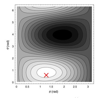
**Fig. 5** Contour plot of the first-order correction  $\Delta F_z^{(-)}$  at  $n_x = 0.8$ ,  $n_y = 0.5$ ,  $n_z = 0.33$  for 3 nm quantum dot. The value of  $\Delta F_z^{(-)}$  rises from dark to light. The cross indicates the donor position
