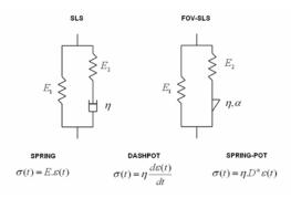
Fig. 1. Standard-linear solid model and the fractional order viscoelastic model.
