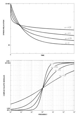
Fig. 2. Time and frequency effects of adjusting the fractional order model  $\alpha$ . Up: Stress-relaxation curves. Down: Complex elastic modulus( $E^*$ ).
