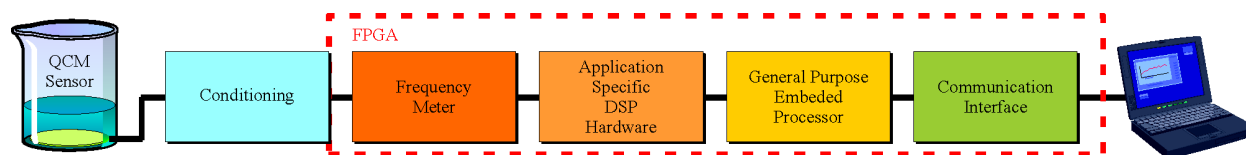
Figure 2. Block diagram of the reconfigurable system for QCM applications.
