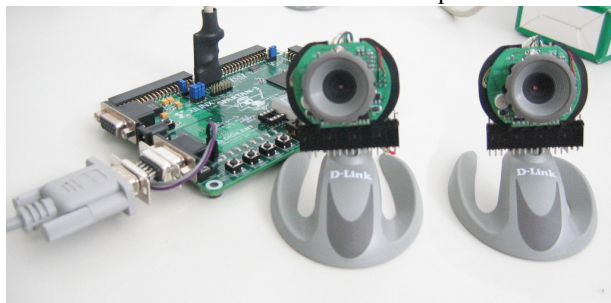
Figure 5. Hardware setup, including the Xilinx FPGA development board and the two CMOS cameras.
