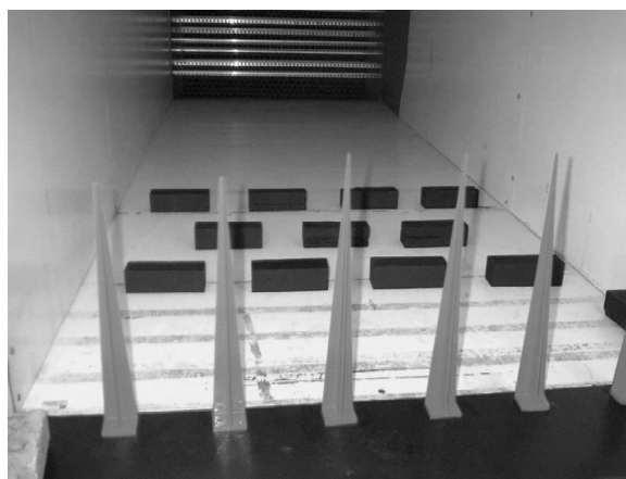
Figure 2. Downstream view of the wind tunnel test section showing the triangular mixing spikes and the roughness elements.
