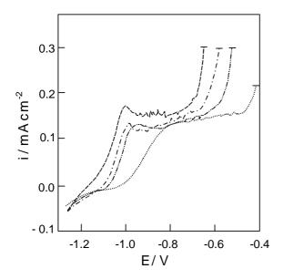
**Fig. 3**: Influence of Cl<sup>-</sup> concentration on the polarization of the In-5%Al alloy.  $v = 0.001 \text{ V s}^{-1}$ .  $E_{s,c} = -1.25 \text{ V}$ . NaCl concentration: (....) 0.01 M; (-..-) 0.1 M; (-..-) 0.5 M; (---) 1.0 M.
