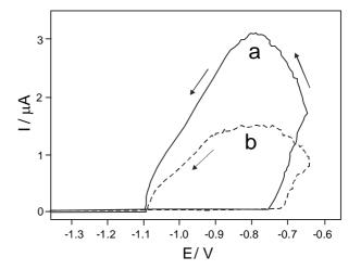
**Fig. 1**: Cyclic voltammetries of Al with and without electrode rotation in 0.5 M LiCl (Dimethylformamide). (a)  $\omega = 0$  rpm; (b) 1800 rpm. V = 0.001 V s<sup>-1</sup>. E<sub>s.a</sub> = -0.63 V, E<sub>s.c</sub> = -1.36 V.
