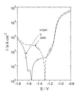
**Fig. 4**: Potentiodynamic polarization of the Al-Zn-In alloy in deareated 0.5 M NaCl solution, pH = 5 with and without electrode rotation. v = 0.001 V s<sup>-1</sup>.  $E_i = -1.8$  V.  $\omega = 2600$  rpm.
