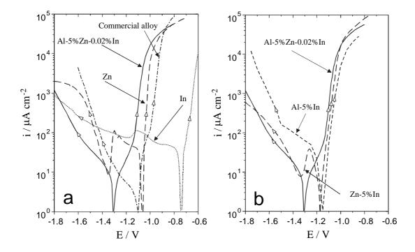
**Fig. 2**: Comparison of the potentiodynamic polarizations of Al-Zn-In with other alloys in areated 0.5 M NaCl solution, pH = 5. (a) Al-Zn-In alloy, commercial Al-Zn-In-Si alloy, Zn and In; (b) binary alloys Zn-5%In and Al-5%In.  $v = 0.001 \text{ V s}^{-1}$ .  $E_i = E_{corr}$ .
