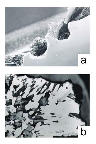
**Fig. 6**: SEM micrograph of an Al-5%Zn-0.02%In alloy after 206 days in sea water: (a) 17X; (b) surface etched with Keller's reagent, 4X.
