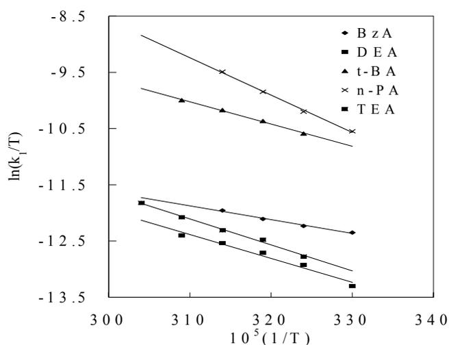
**Fig. 3.** Eyring plots of  $\ln(k_1/T)$  vs.  $1/T$  for the reaction of different bases with  $\text{trans-}[\text{Co}(\text{en})_2\text{Cl}_2]^+$  in DMA solution.
