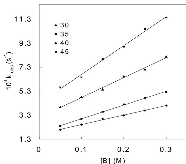
**Fig. 1.** The plots of  $k_{\text{obs}}$  vs.  $[n\text{-propylamine}]$  in DMA solution at  $\mu = 0.80 \text{ M}$  and different temperatures.
