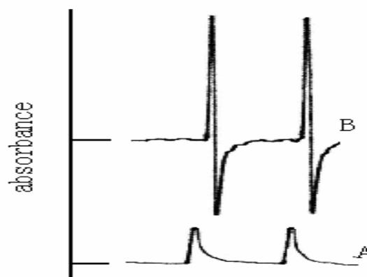
**Fig. 3.** Absorption signal of conventional (A) and derivative (B) FI-FAAS.
