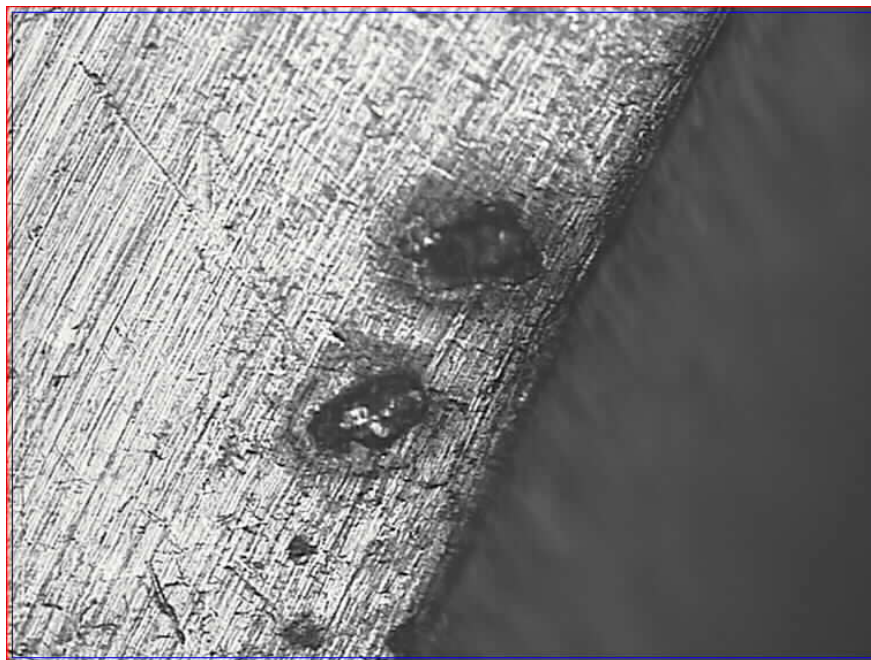
Figure 2. The well-grown pits observed on the bent region of the 316SS U-bend specimen exposed to deaerated 0.5M NaCl solution during EN experiment.
