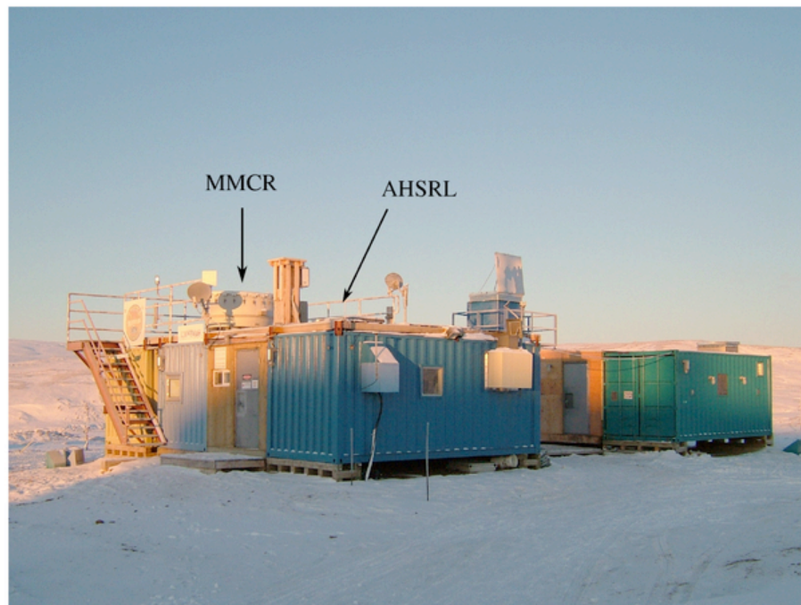
Fig. 2. A photograph of the Zero-altitude PEARL Auxiliary Laboratory (ØPAL) with pointers to the Arctic High Spectral Resolution Lidar (AHSRL) and Millimeter-wave Cloud Radar (MMCR) locations.
