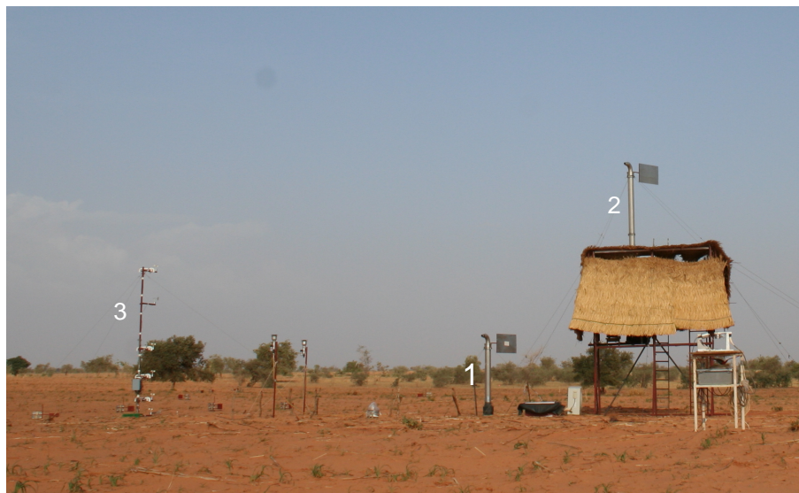
Fig. 1. View of the experimental site showing the two sampling systems located at elevations of 2.1 m above the buried container (1) and of 6.5 m on the tower (2), and the meteorological mast (3).
