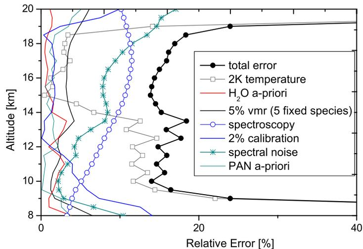
**Fig. 10.** Estimated total and individual relative errors in  $\text{PAN}_{\text{MIPAS-STR}}$  analysis.
