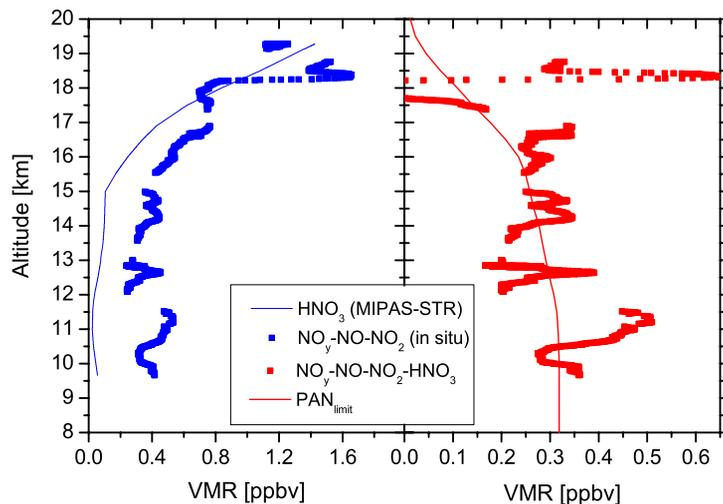
**Fig. 2.** Comparison of  $\text{HNO}_3$  from MIPAS-STR with in situ measured  $\text{NO}_y\text{-NO-NO}_2$  (left) and the difference of  $\text{NO}_y\text{-NO-NO}_2\text{-HNO}_3$  (right). In the right panel we give also the smoothed difference used in Sect. 4.6.
