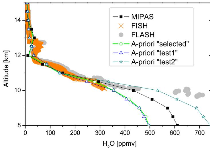
**Fig. 5.** The retrieved  $\text{H}_2\text{O}$  profile (simultaneously fitted with  $\text{PAN}_{\text{MIPAS-STR}}$ ) and the selected a priori profile are shown together with in situ data from the FLASH and FISH instruments and two modified a priori profiles ( $\text{test}_1$ ,  $\text{test}_2$ ), used for error estimation.
