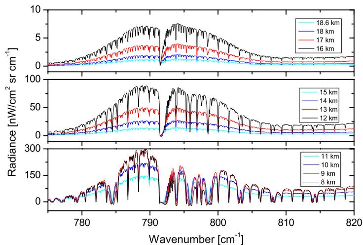
**Fig. 4.** Simulated difference spectra (with – without PAN) in the broad-band range of PAN for all tangent heights from 8 to 18.6 km. The noise level of MIPAS-STR is about  $15 \text{ nW}/(\text{cm}^2 \text{ sr cm}^{-1})$ .
