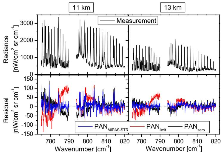
**Fig. 9.** MIPAS-STR measured spectra in black (top panels) and the residual spectra (forward calculation – measurement) in blue, red and black of  $\text{PAN}_{\text{fit}}$  and the tests  $\text{PAN}_{\text{limit}}$  and  $\text{PAN}_{\text{zero}}$  (lower panels) at tangent heights of 11 km (left panels) and 13 km (right panels).
