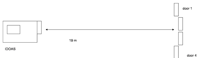
Fig. 5. Ground setup used to characterise the optical properties of the airborne iDOAS. Each hangar door was 4.5 m wide and the small openings in between were 30 cm, hence the total distance between the light sources was 9.9 m (edge to edge).
