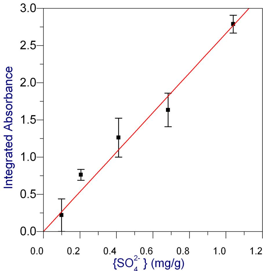
Fig. 7. Calibration curve for the integrated absorbance versus the concentration of sulfate.
