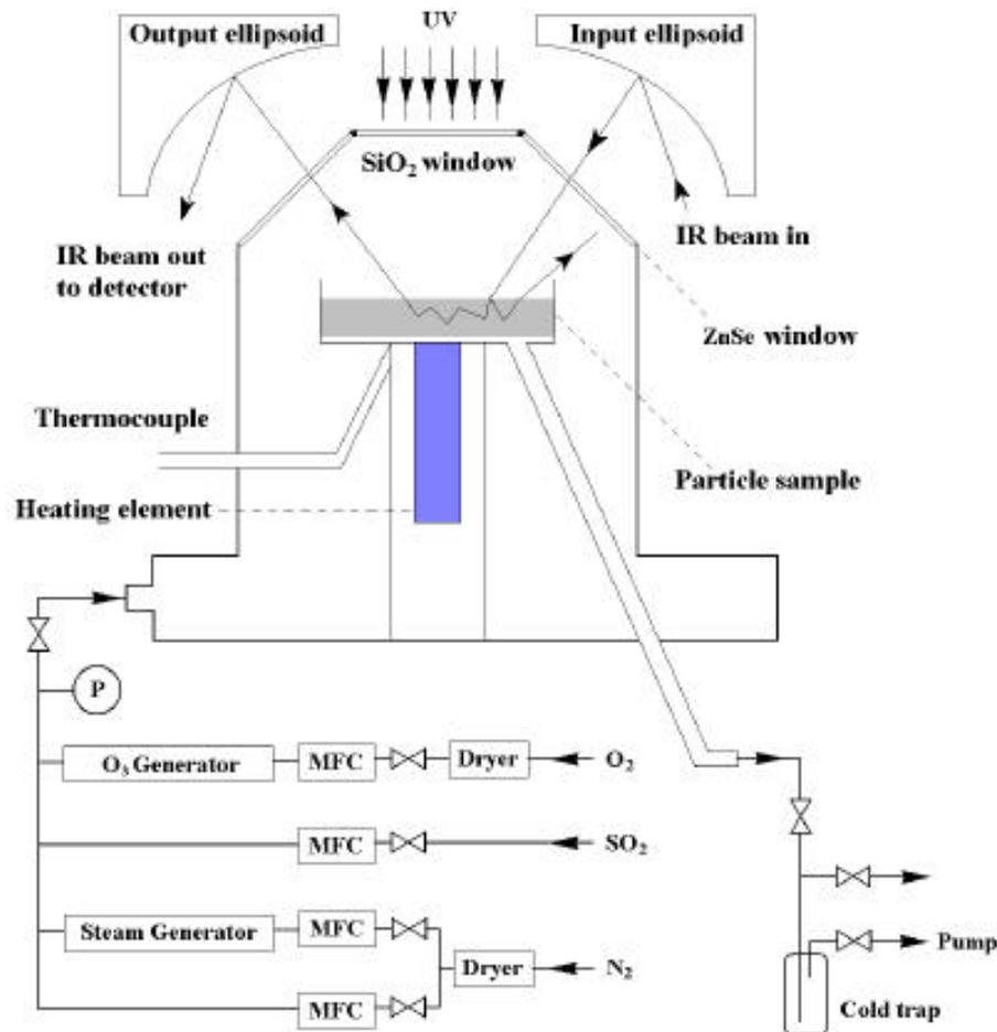
**Fig. 1.** Schematic diagram of the experimental set-up including the DRIFTS apparatus, the O<sub>3</sub> generator, steam generator, pressure gauge (P), mass flow controller (MFC), silicon and zeolite dryer, cold trap, pump and mixing lines.
