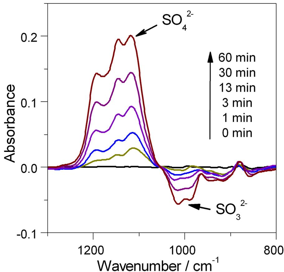
**Fig. 3.** In situ DRIFTS spectra of O<sub>3</sub> oxidation of sulfite mixed into CaCO<sub>3</sub> powder. The unexposed sample was used to collect a background spectrum and the sulfate positive band at 1100 cm<sup>-1</sup> and the sulfite negative band at 1000 cm<sup>-1</sup> changed with the reaction time.
