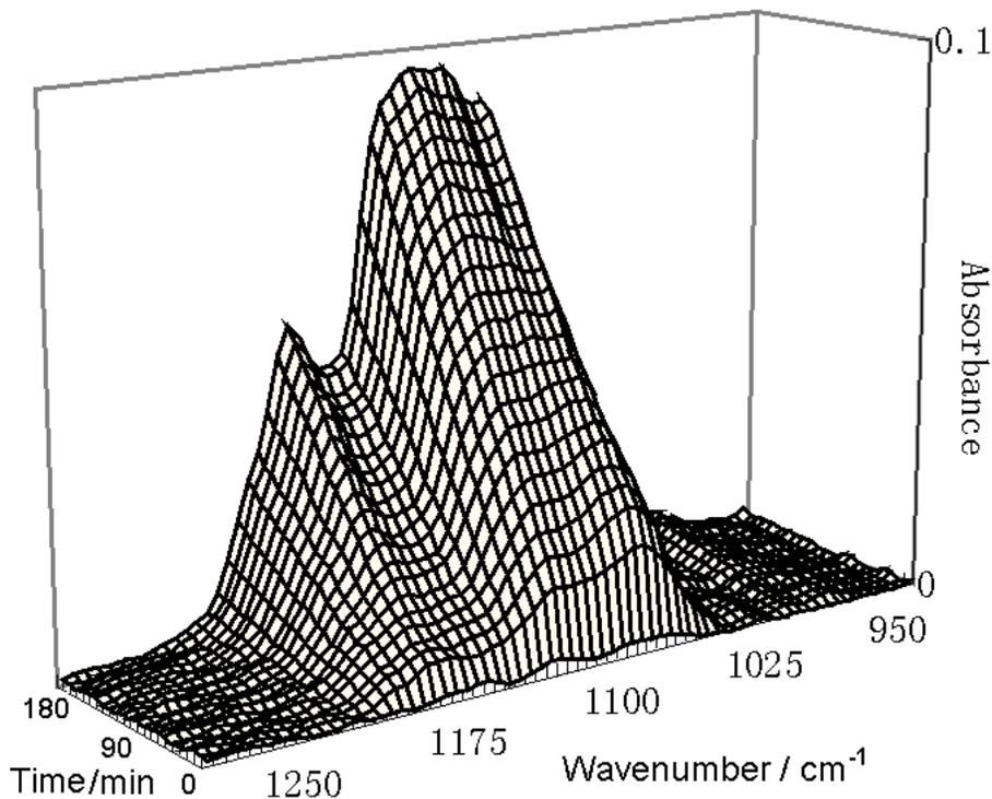
**Fig. 4.** Absorption bands observed during the reaction of SO<sub>2</sub> with O<sub>3</sub> on the surface of CaCO<sub>3</sub> as a function of reaction time ([SO<sub>2</sub>]=4.92×10<sup>14</sup> molecules cm<sup>-3</sup>, [O<sub>3</sub>]=4.92×10<sup>14</sup> molecules cm<sup>-3</sup>).
