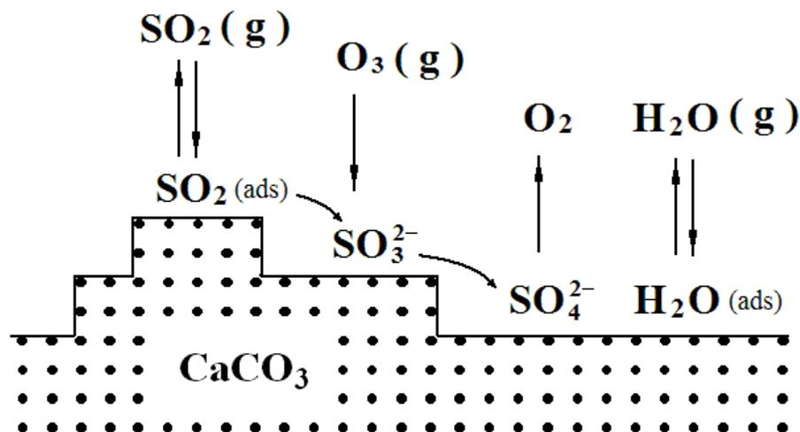
**Fig. 10.** Schematic diagram of the mechanism of  $\text{SO}_2$  oxidation by  $\text{O}_3$  on  $\text{CaCO}_3$  surface. Gas-phase  $\text{SO}_2$  can be adsorbed on the surface. At the same time, water vapor can be reversibly adsorbed on surface. Under the cooperation of adsorbed water and the basicity given by  $\text{CaCO}_3$ , adsorbed  $\text{SO}_2$  is transformed into sulfite, and then the sulfite is rapidly oxidized into sulfate by  $\text{O}_3$ .
