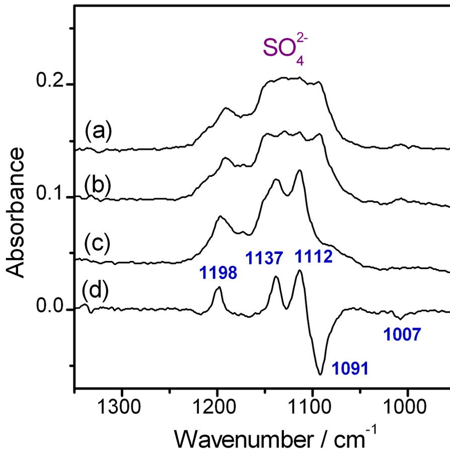
**Fig. 5.** Spectra of sulfate when the reactor with the sample was evacuated and heated. **(a)** Sample after a typical experiment with  $\text{SO}_2$  and  $\text{O}_3$  exposure, followed by evacuation to 10 Pa **(b)** and, further heating to 300°C **(c)**; **(d)** difference between the spectrum (a) and (c).
