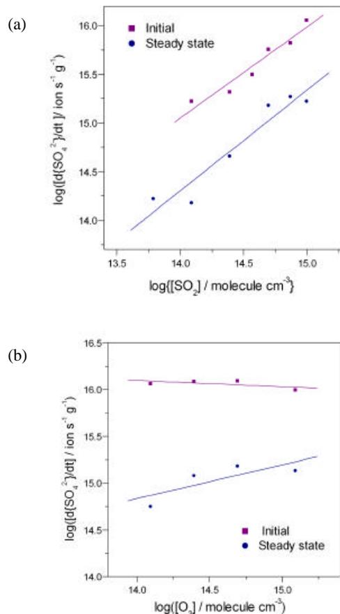
**Fig. 8.** Double-logarithmic plot of the rate of sulfate formation as a function of  $[\text{SO}_2]$  and  $[\text{O}_3]$  at initial time and steady state. The reaction order in  $\text{SO}_2$  was determined from a linear regression yielding  $n_0=0.94\pm 0.06$  ( $\sigma$ ),  $n_{ss}=1.04\pm 0.13$  ( $\sigma$ ). For  $\text{O}_3$  corresponding values are  $n_0=0.06\pm 0.26$  ( $\sigma$ ),  $n_{ss}=0.36\pm 0.45$  ( $\sigma$ ).
