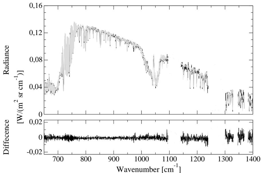
**Fig. 5.** Comparison of REFIR-PAD and IASI-balloon measurements (top panel – black and grey lines, respectively) and differences (bottom panel) in the common spectral region. Measurements were acquired near the end of flight at 14:49 UTC.
