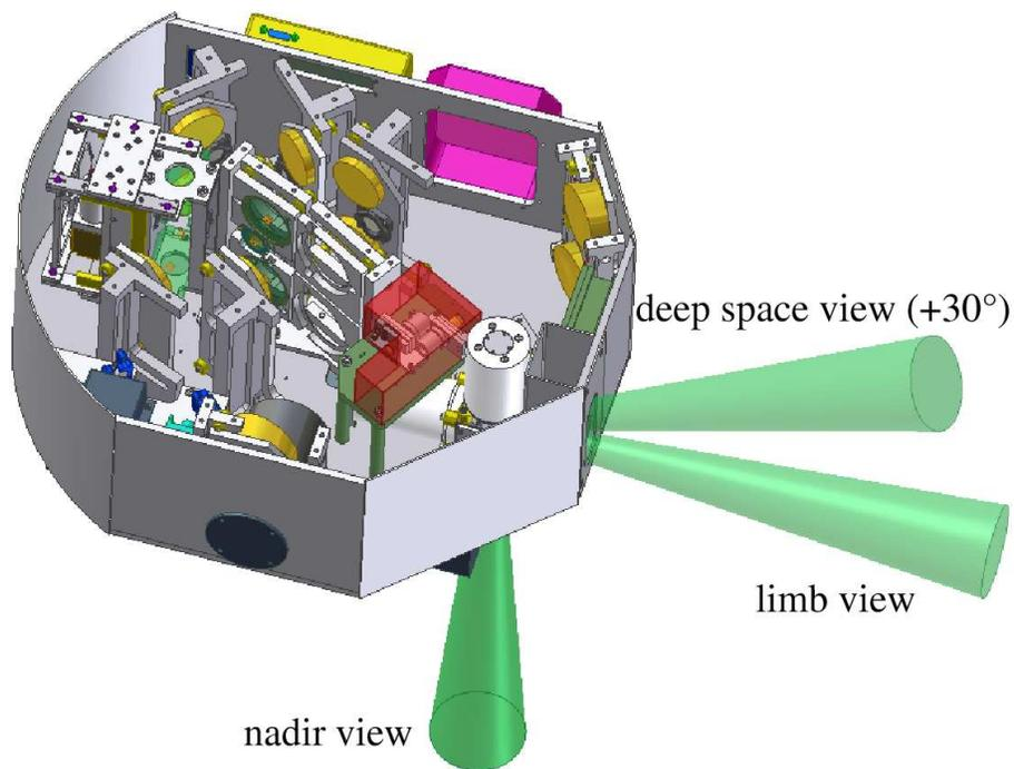
**Fig. 1.** REFIR-PAD illustration with three different viewing directions.
