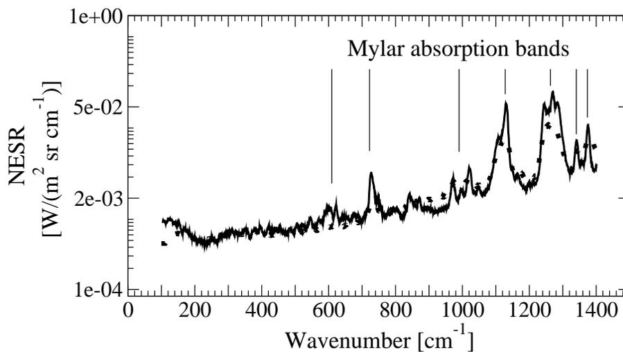
**Fig. 2.** Comparison between NESR measured during the 30 June 2005 flight (solid line) and lab vacuum tests (dots).
