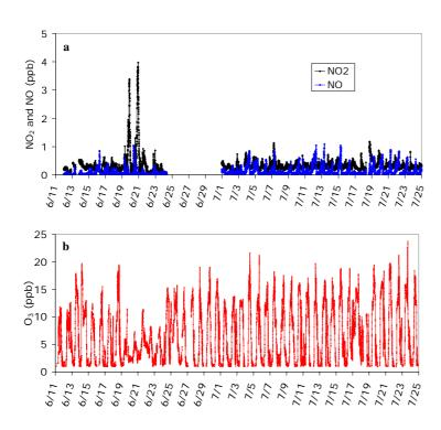
**Fig. 7.** Time series of **(a)** NO and NO<sub>2</sub> and **(b)**  $O_3$  concentrations (ppb) measured from 12 June to 25 July 2001 during LBA-CLAIRE 2001.
