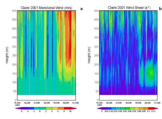
Fig. 5. Time series of (a) meridional wind and (b) wind shear from SODAR during LBA-CLAIRE 2001.
