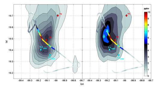
Fig. 6. Comparison between toluene mixing ratios measured during RF8 and modeled with WRF-Chem using CAM 2001 (left panel) and the adjusted CAM 2004 (right panel) emission inventory during the C-130 MCMA flight segment.
